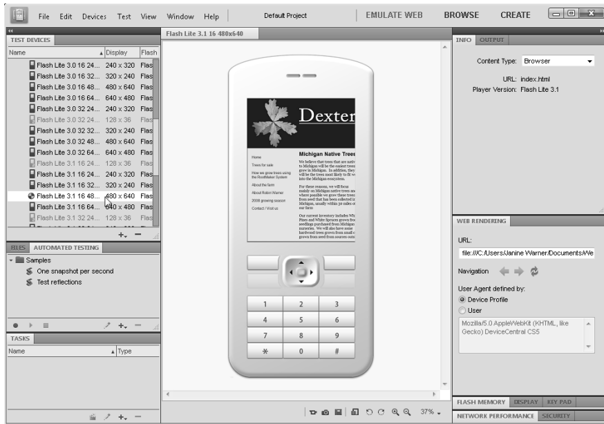
Figure 4-6: Adobe Device Central makes it possible to view your Web pages as they will appear in a variety of mobile devices.
