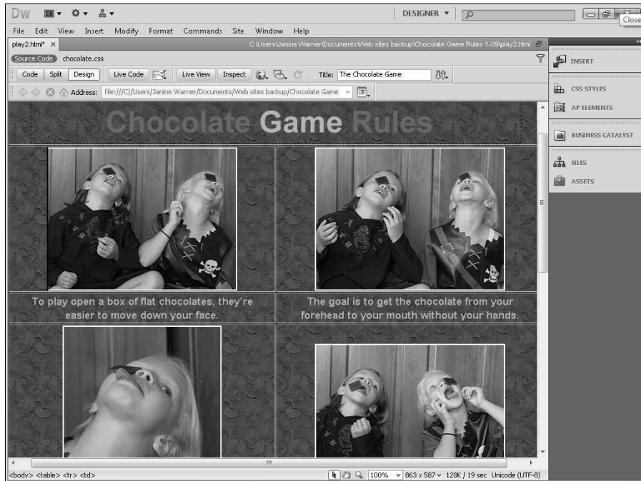
Figure 8-9: Many two-column page layouts, such as the one shown here, were created with HTML tables.
