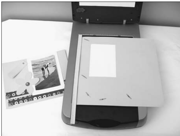
Figure 18-1: A thin piece of wood can be used to position a page properly on the scanner.
