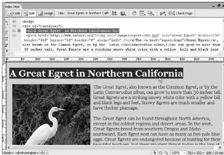
Figure 3-4: The Split view option in Dreamweaver makes it possible to display in the workspace both the page design and the code behind the page.
