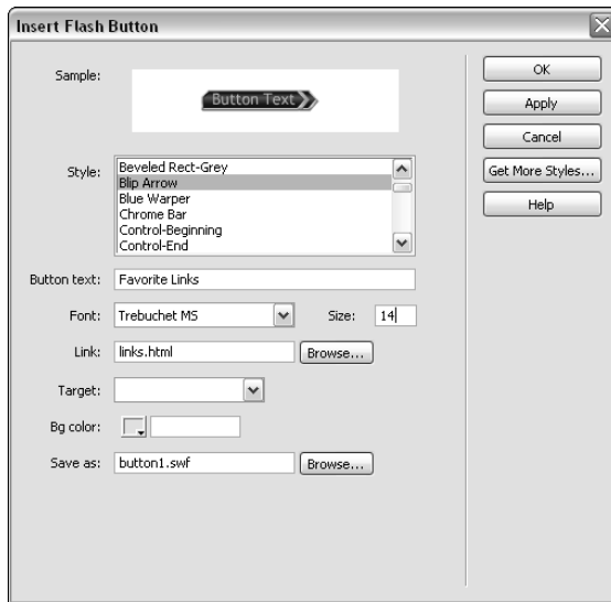
Figure 11-3: The Insert Flash Button dialog box lets you create and edit interactive Flash button graphics within Dreamweaver.
