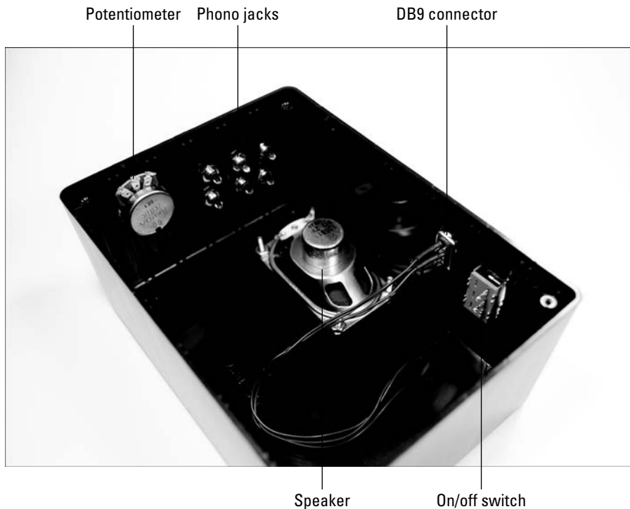
Figure 7-11: Mount components on the box.
