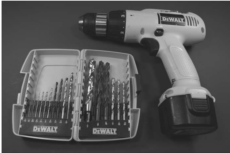
Figure 3-2: A \frac{3}{8} " drill and an assortment of drill bits.
