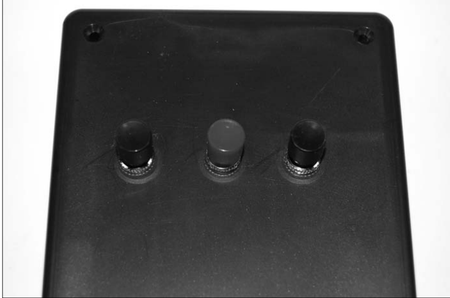
Figure 11-16: Transmitter box with switches installed.
