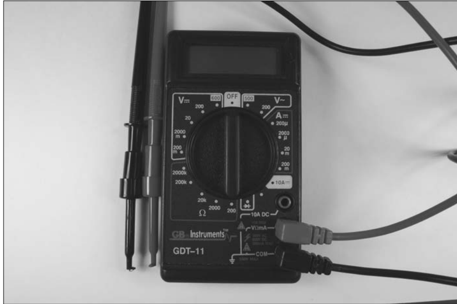
Figure 1-3: A multi- meter is a measuring device that you'll use often.
