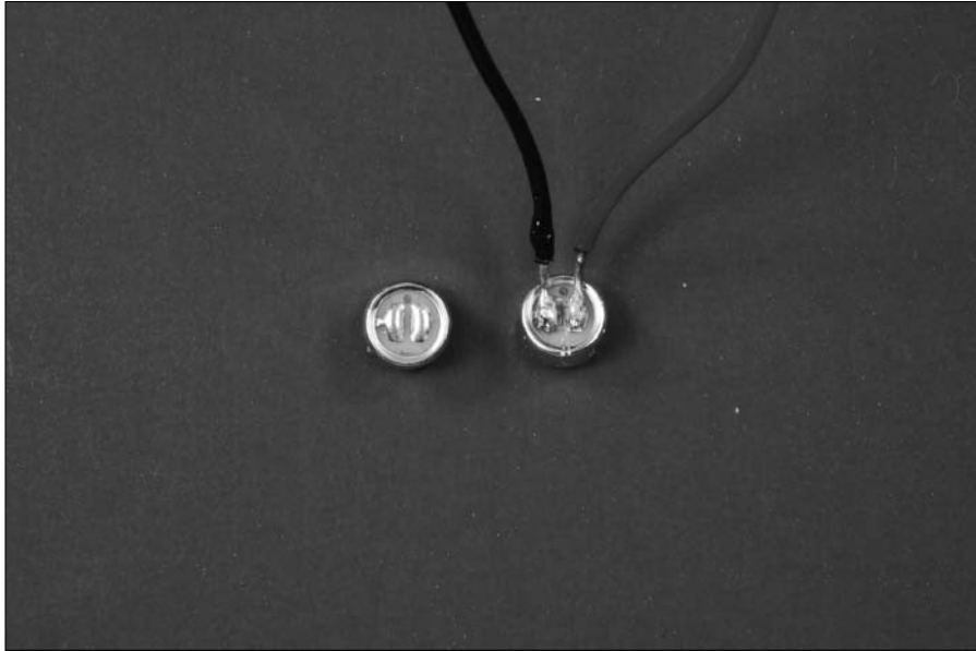
Figure 4-14: Soldering to flat contact pads.
