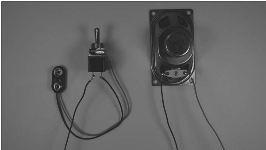
Figure 9-23: Wires soldered to speaker and on/off switch.
