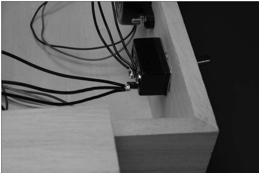
Figure 13-35: Wires soldered to on/off switch.
