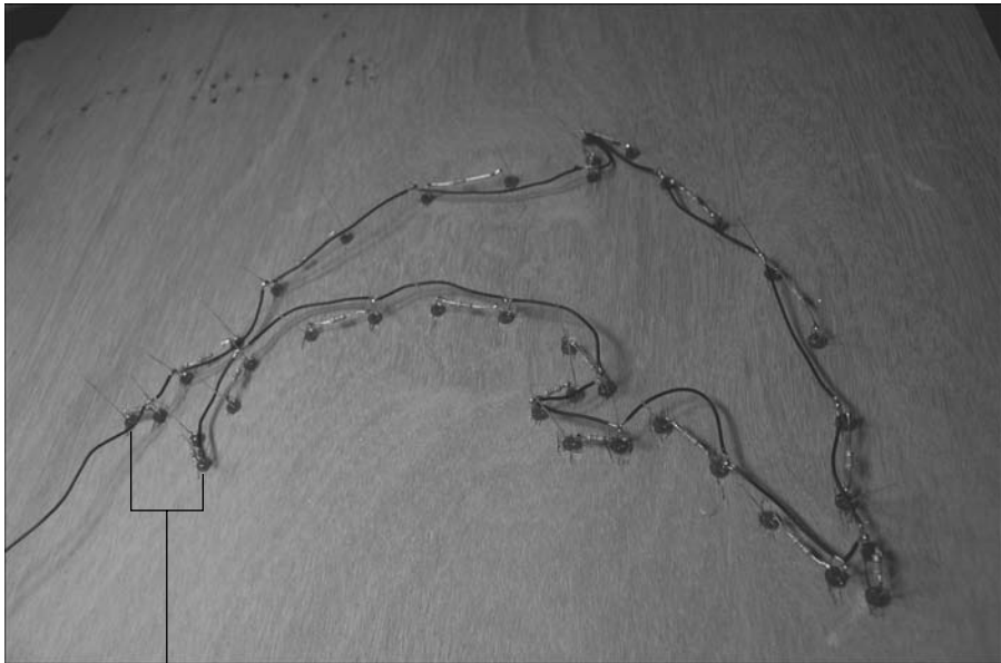
Figure 10-18: Black wires connecting short leads of LEDs.
