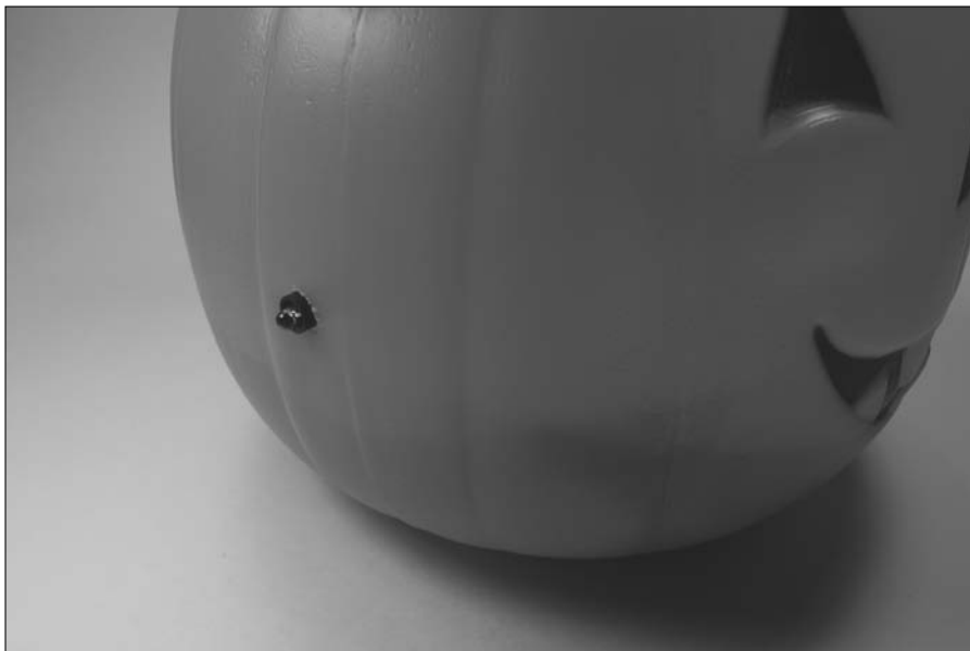
Figure 9-17: Silent pumpkin with LED socket installed.
