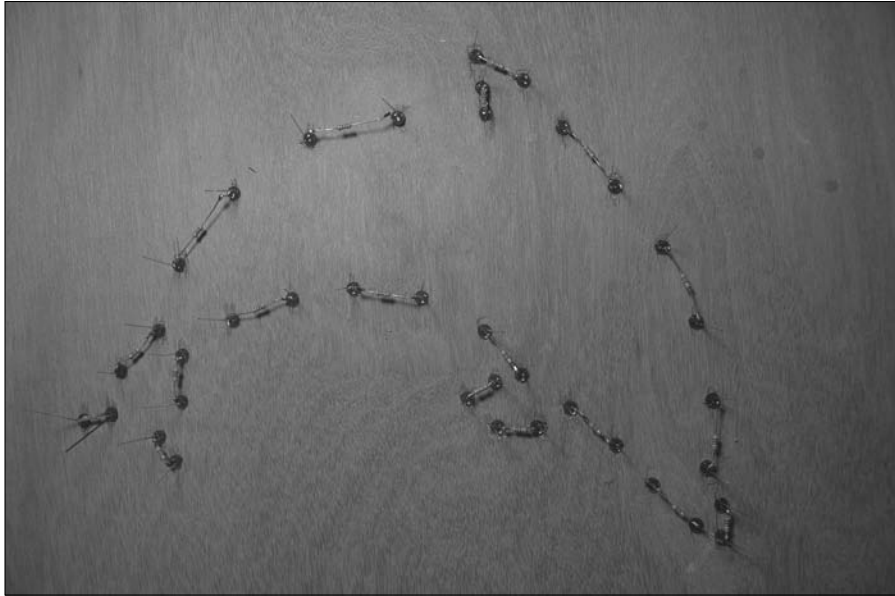
Figure 10-17: Resistors soldered and leads clipped.
