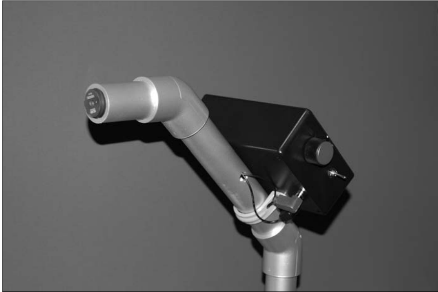
Figure 12-18: The finished metal detector.
