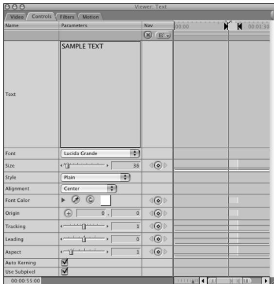
Figure 13-2: You can change attributes for the Text text generator on the Controls tab in the Viewer window.
