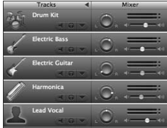
Figure 10-4: Drums and vocals are panned dead center, harmonica and guitar are panned hard right and left, and bass is panned soft right.
