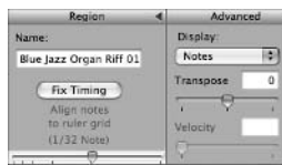
Figure 9-6: You can change the pitch of your loop by moving the Transpose slider to the right or the left, or by typing a new value in the Transpose field.
