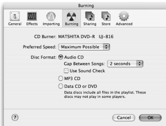
Figure 12-5: iTunes' Burning pane should look like this when you're ready to burn an audio CD.
