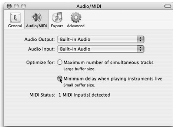
Figure 16-7: Optimize for recording (as shown) or mixing (choose large buffer size) on this tab.
