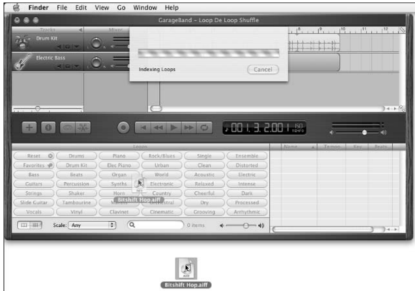
Figure 5-7: Drag the loop file from the Finder and drop it into the Loop Browser to add it to your personal loop library.
