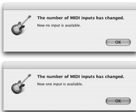
Figure 3-7: GarageBand politely informs you every time that a MIDI device is disconnected (top) or connected (bottom). Sweet!
