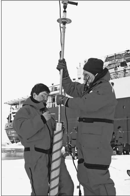
Figure 3-2: Drilling for an ice core sample.
