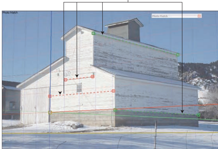
Color Plate 12: All four Perspective bars, properly lined up with edges in the picture (Chapter 7).
