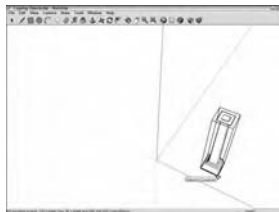
Figure 2-25: To make multiple copies in a row, type in the number of copies you want, type an x and press Enter.
