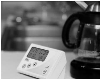
Figure 13-3: Gauge your home's total energy usage in real time.
