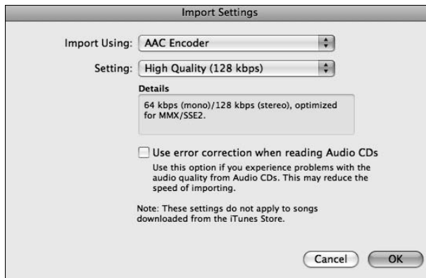
Figure 4-10: Ripping a CD with battery- friendlier settings.
