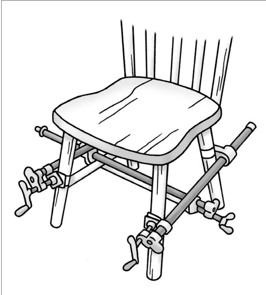
Figure 20-2: Use flexible clamps or several rigid bar clamps to hold the repaired chair rungs.
