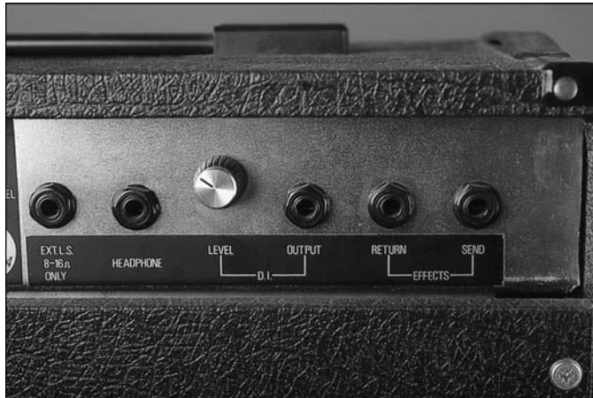
Figure 2-7: With an effects loop, you can route signals out for processing and then back in.
