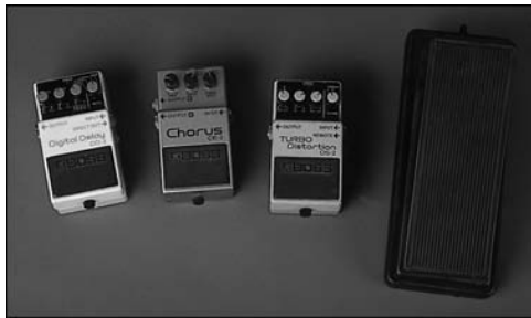
Figure 1-3: Four common effects (left to right): digital delay, chorus, distortion, wah-wah.
