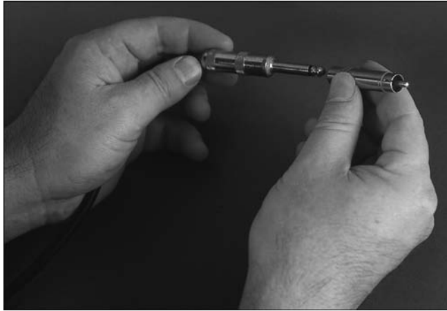
Figure 2-11: An adapter allows you to use your stereo or boombox as an amp.
