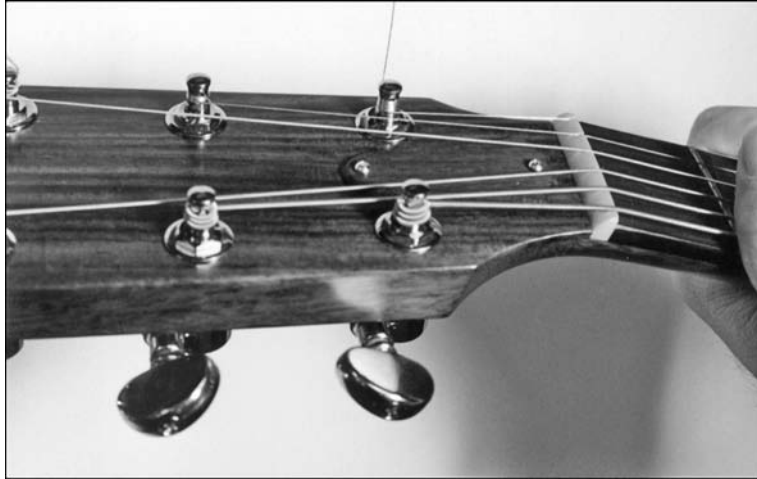
Figure 3-5: The treble strings wrap downward around the posts in a clockwise direction; the bass strings wrap around the posts in a counterclockwise direction.
