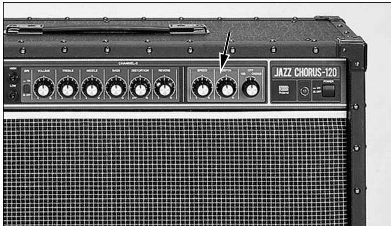
Figure 2-6: The two controls that modify the chorus here are speed and depth .
