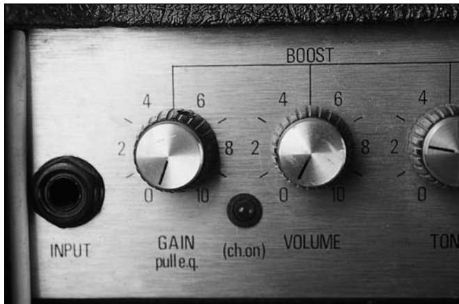
Figure 2-3: A tale of two volumes: preamp and power amp, channel, and master.
