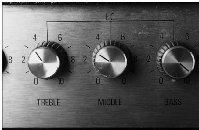
Figure 2-4: The tone controls of an amp's EQ, or tone-shaping, section.
