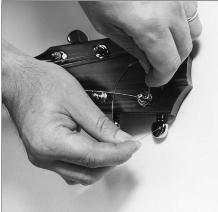
Figure 3-4: String kinked to the inside of the head- stock, with slack for winding.
