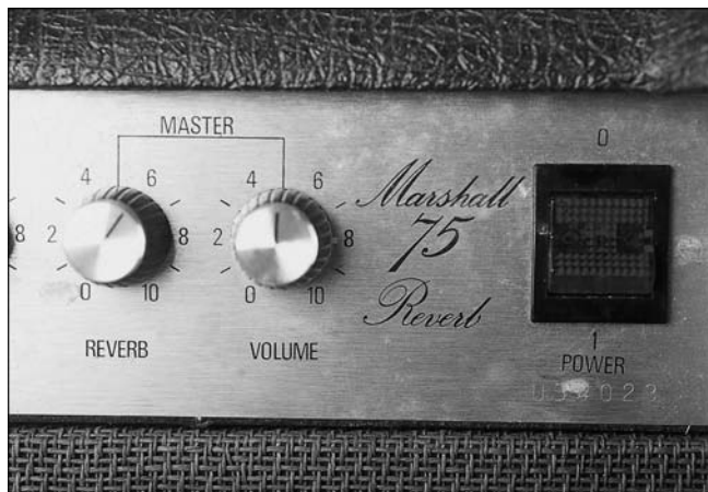
Figure 2-5: The control for amp reverb is usually limited to one knob.
