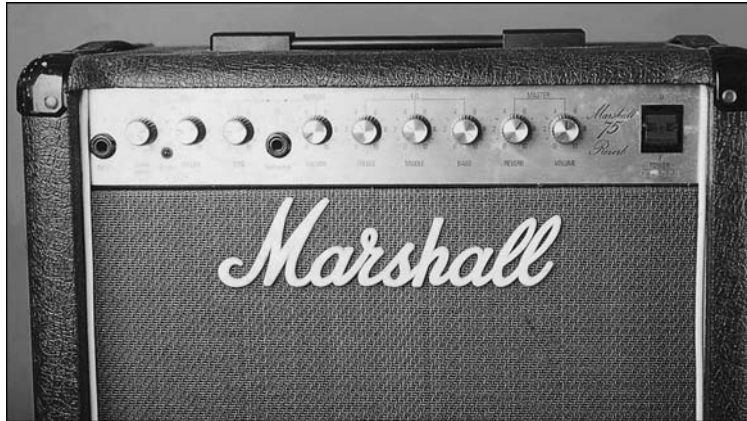
Figure 2-2: The control panel groups an amp's jacks, switches, and knobs.
