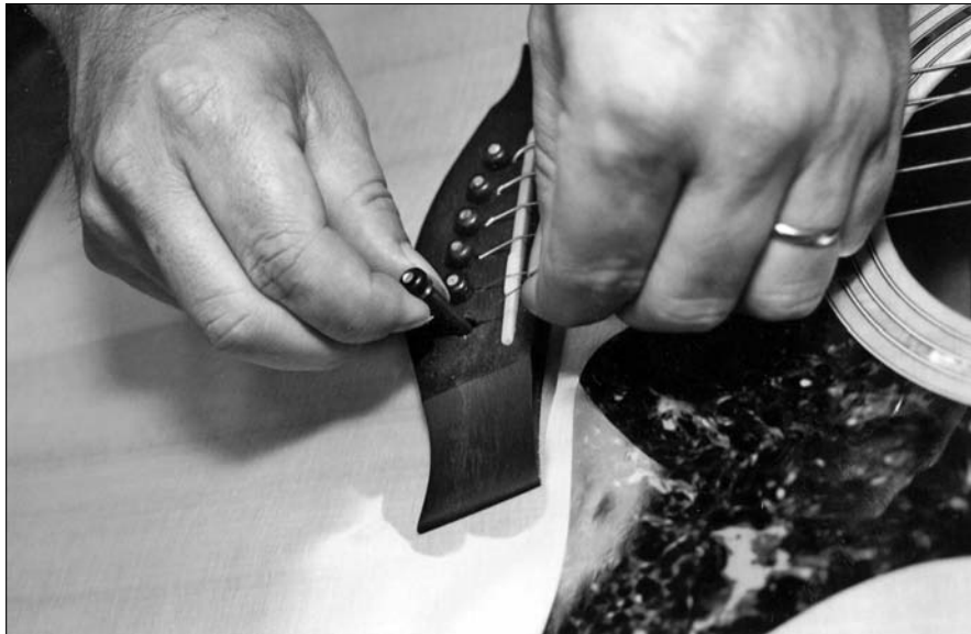
Figure 3-3: How to place the new string in the bridge and position the bridge pin.
