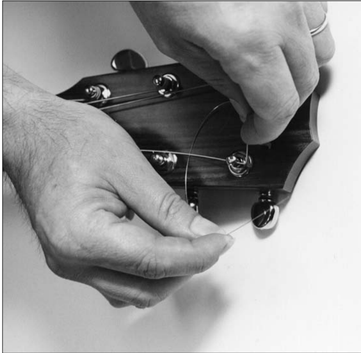
Figure 17-2: String kinked to the inside of the headstock, with slack for winding.
