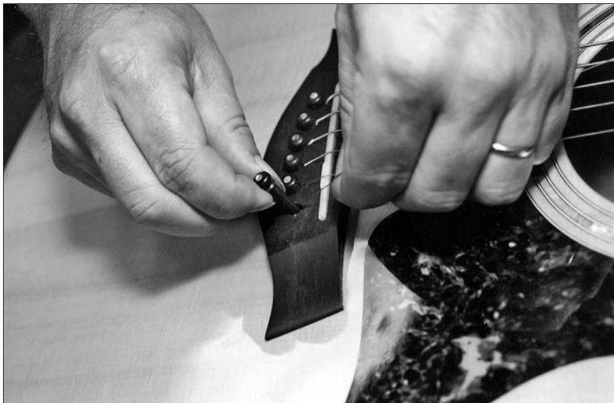
Figure 17-1: How to place the new string in the bridge and position the bridge pin.
