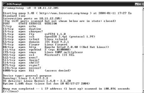
Figure 12-5: Using Nmap to determine the OS kernel version of a Linux server.
