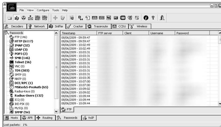
Figure 7-8: Using Cain & Abel to capture passwords going across the network.
