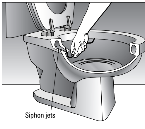
Figure 8-1: Clearing clogged siphon jets.
