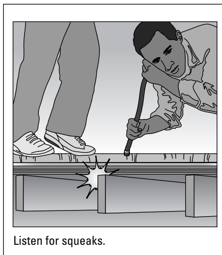
Figure 4-7: Finding floor squeaks.
