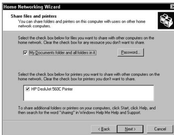
Figure 6-8: The wizard assumes you want to share your documents folder and any printer that's connected to this computer.
