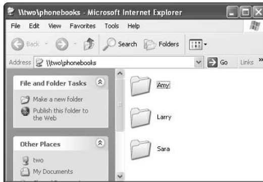
Figure 11-7: Use your browser to access shares, and add oft-used UNC's to your Favorites list.
