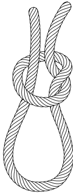
Figure A-6: Use a slip knot to temporarily hold something in place.
