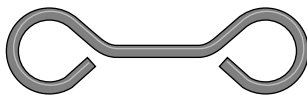
Figure 7-31: Bend the loops to move the crossbar to the center of the component.
