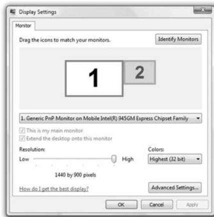
Figure 2-1: The standard set of controls offered by Windows allows you to select resolution and high or medium levels of colors, as well as other settings.
