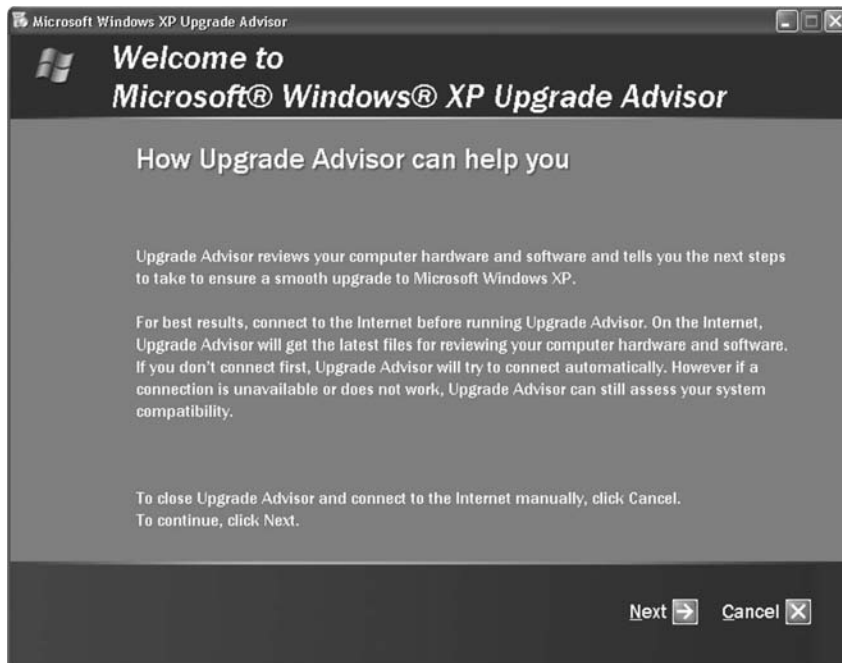
Figure 1-3: Microsoft's Windows XP Upgrade Advisor, a free utility, examines your machine to see if installed hardware and software are upgrade candidates.
