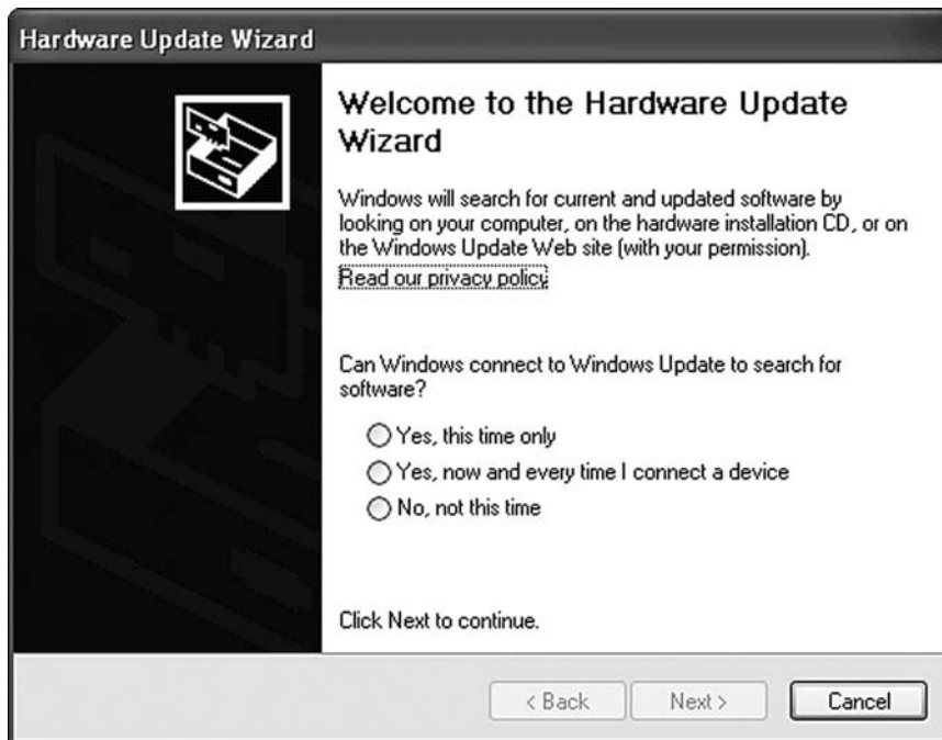
Figure 3-7: The Windows XP version of the Hardware Update Wizard checks for newer versions of device drivers installed in your machine.
