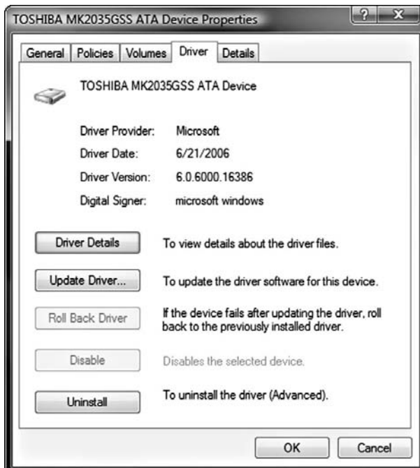
Figure 1-4: The Driver tab includes a button to update the driver manually. You're asked for the new driver's location.
