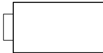
Figure 2-7: A version of the symbol for a battery is used by laptop makers to indicate that the machine is running on its own battery-stored energy.
