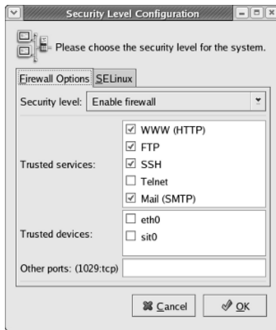
Figure 3-2: In Fedora Core, you can set up packet filtering with this tool.
