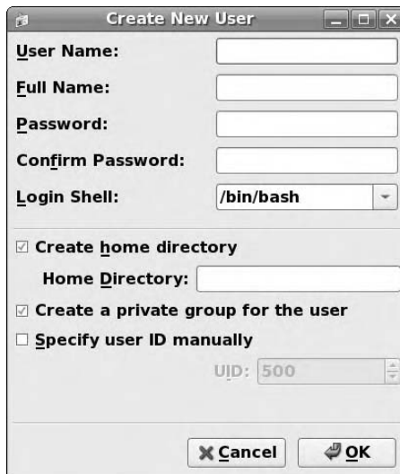
Figure 7-2: The Create New User dialog box in the User Manager application, in Fedora Core 5.
