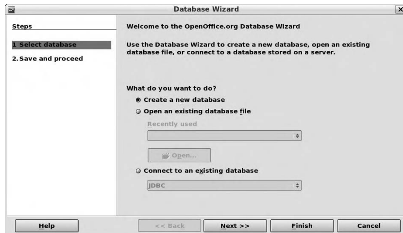
Figure 17-6: The OpenOffice.org Base Database Wizard, used to open existing databases and create new ones.
