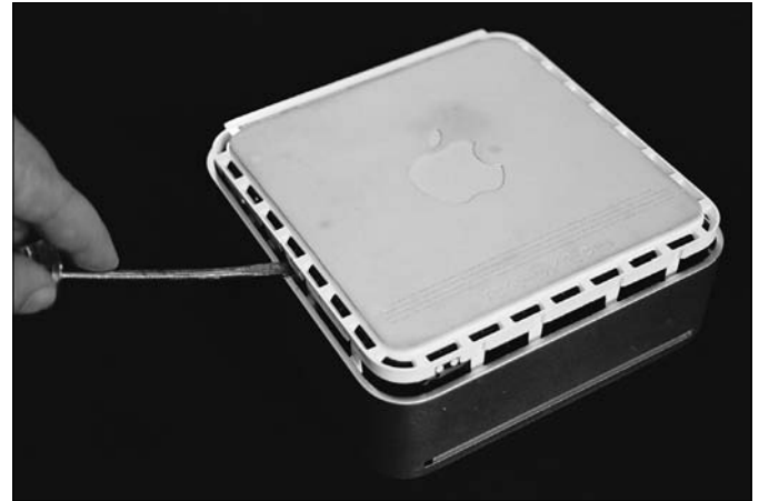
Figure 22-5: Carefully prying the plastic base out
