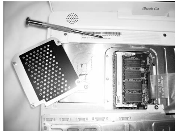
Figure 22-3: A RAM slot under the keyboard
