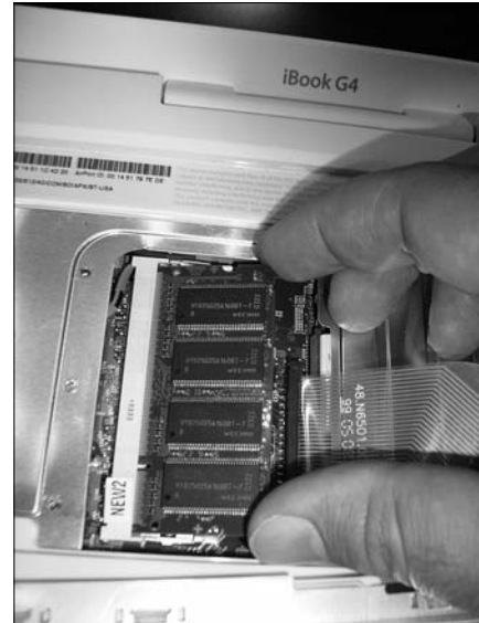
Figure 22-4: Seating the RAM and securing the retention clips
