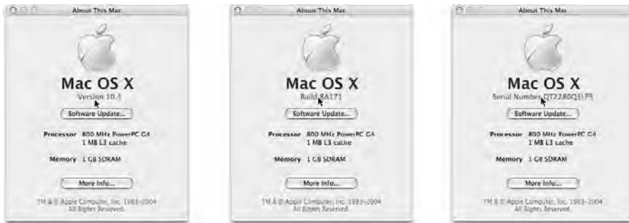
Figure 3-13: Click the version, build, or serial number to cycle through these three variations of About This Mac.
