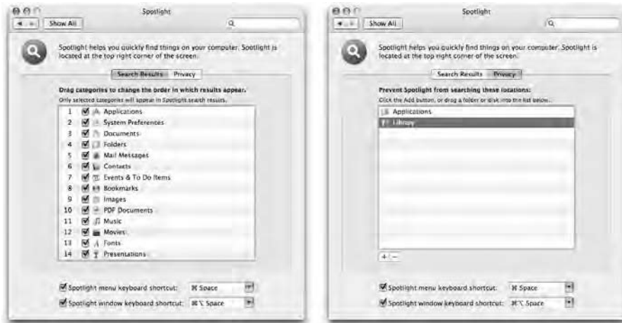
Figure 13-11: Search Results lets you specify which results get shown in what order and Privacy lets you specify which locations not to search.
