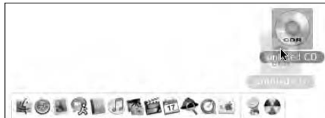
Figure 7-3: Just drag the disk icon to the Burn Disc (with a c ) button on the Dock when you're ready to burn your CD.
