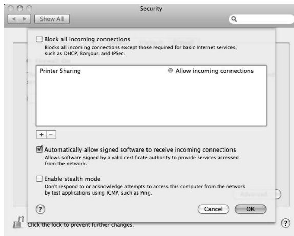
Figure 2-2: You can help protect your MacBook by using Snow Leopard's built-in firewall.
