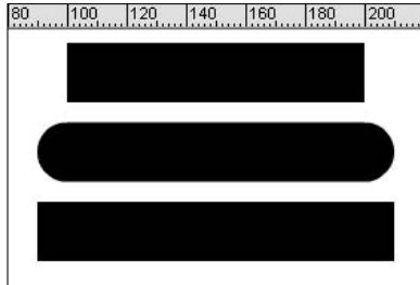
Figure 3-4: These three lines were all drawn to be 100 pixels long, but the bottom two lines have round and square caps, so they're longer.
