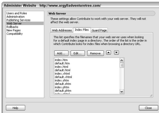
Figure 3-5: Contribute looks for pages on the server in the order the filenames appear in the Index Files list.
