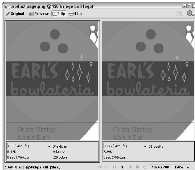
Figure 6-8: Comparing two possible compression settings side by side in the 2-Up view.
