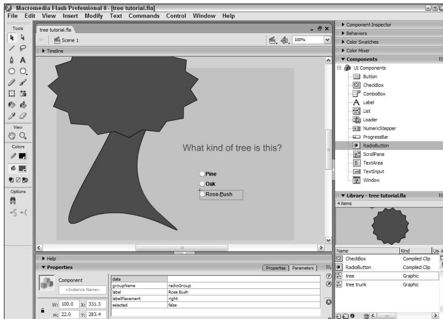
Figure 9-2: The Properties panel when a radio button component is selected.
