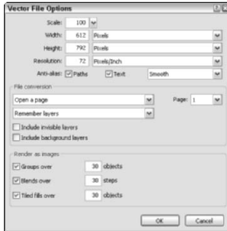
Figure 8-5: The Vector File Options dialog box allows you to set various options when you import a FreeHand file into Fireworks.
