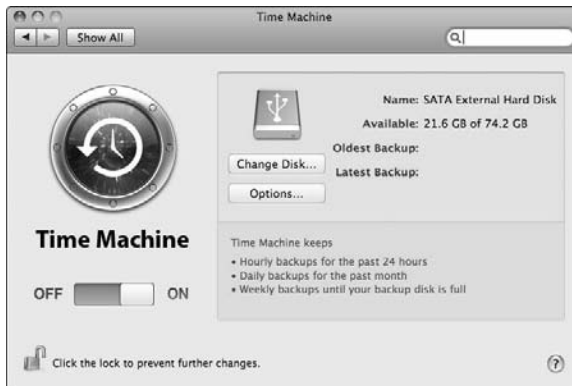
Figure 1-3: The Time Machine pane can show how much free space remains on your external hard drive.
