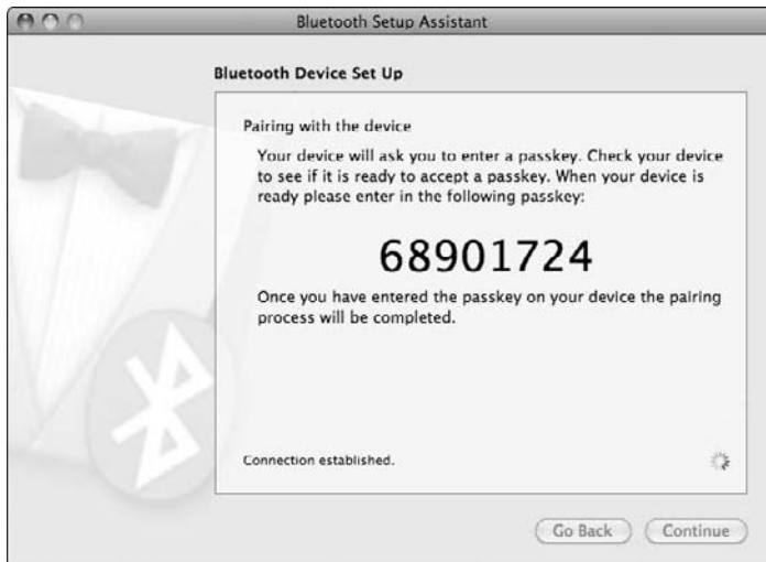
Figure 3-5: The Bluetooth dialog offers to define a passkey for linking another device to your Mac.
