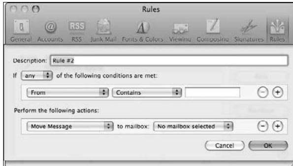
Figure 2-21: Clicking different pop-up menus lets you define a rule for routing your messages.
