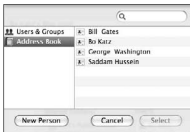
Figure 2-4: A dialog lets you create a new user who can access your shared folder.
