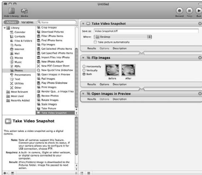
Figure 5-10: Three actions that take your picture, flip it upside-down, and then display it on the screen.
