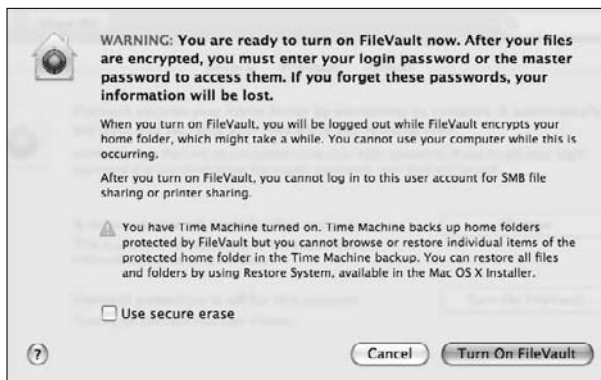
Figure 1-9: A warning dialog appears to let you know the consequences of using FileVault.
