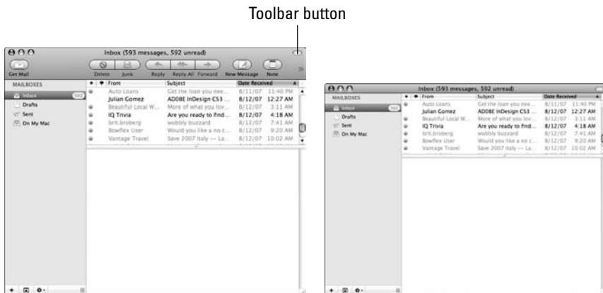
Figure 3-13: The Toolbar button can display (left) or hide (right) a window's toolbar.
