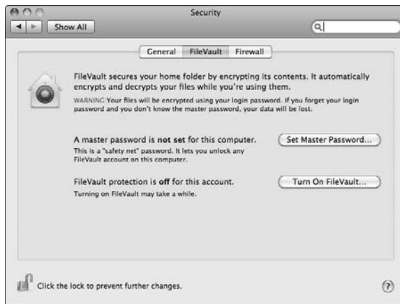
Figure 1-7: The FileVault pane lets you turn on FileVault and set a password.
