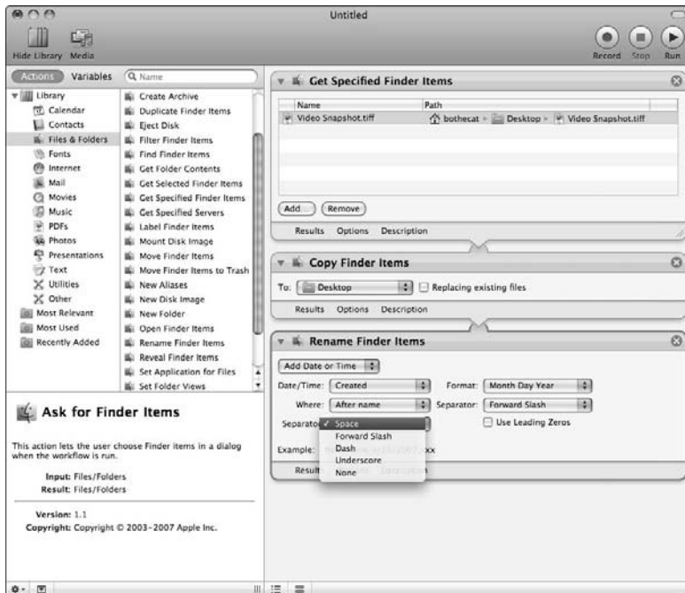
Figure 5-14: The Rename Finder Items action displays pop-up menus for defining how to name a file.
