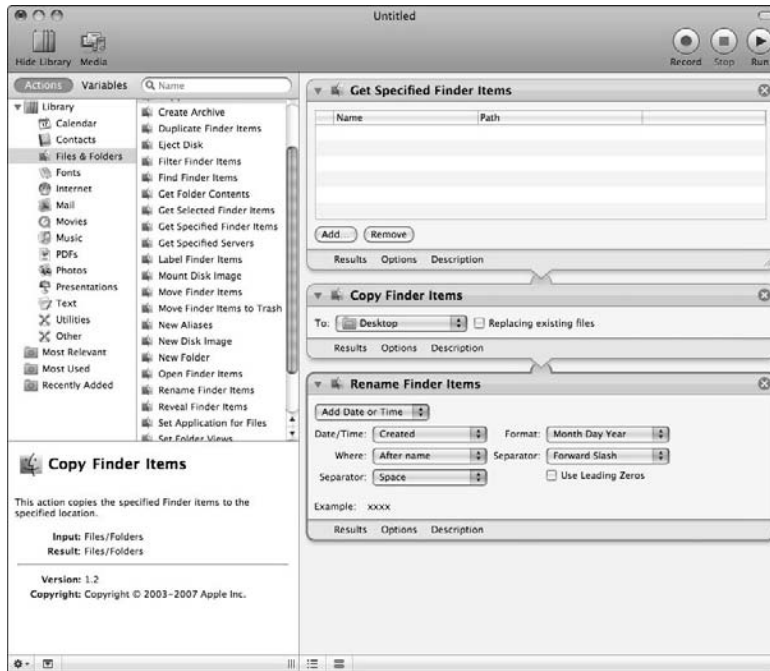
Figure 5-12: Three actions that take a file, copy the file to the Desktop, and then rename that copy of the file.
