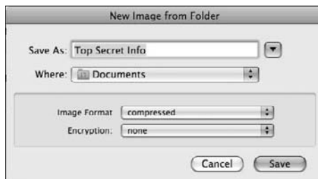
Figure 6-18: A dialog appears where you can name and define the location of your disc image file.
