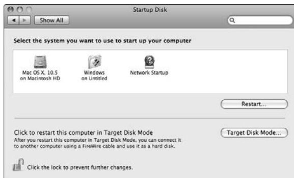
Figure 4-5: The Startup Disk window lets you choose which partition to make the default startup disk.
