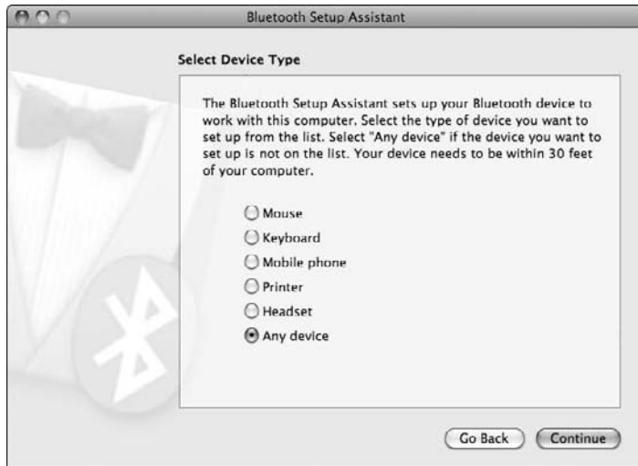
Figure 3-3: The Bluetooth Setup Assistant dialog lets you define the type of Bluetooth device to pair with your Mac.
