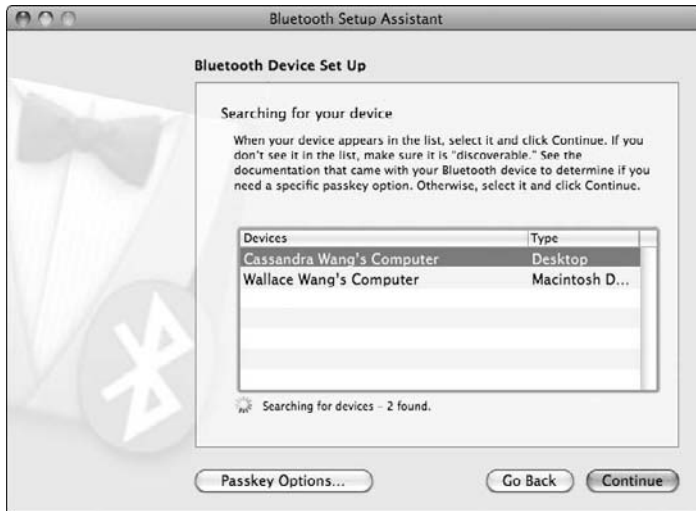
Figure 3-4: The Bluetooth dialog lists all Bluetooth-enabled devices that you can pair with your Mac.
