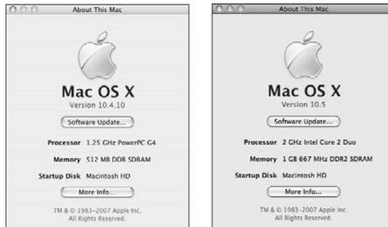
Figure 1-1: The About This Mac window identifies the processor used in your Mac.
