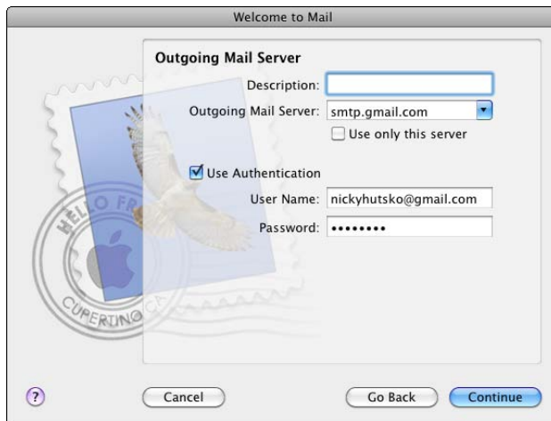
Figure 2-3: The Outgoing Mail Server asks for the name of the server to send your e-mail through to the rest of the Internet.
