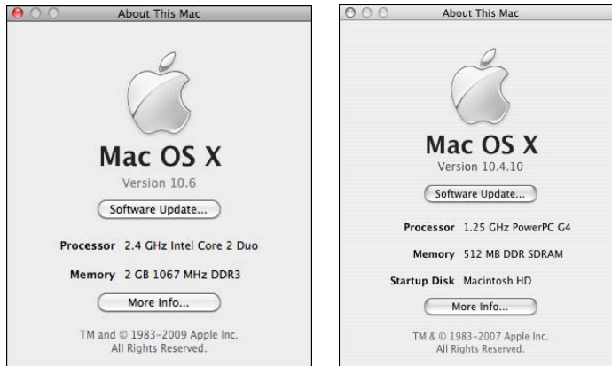
Figure 1-1: The About This Mac window identifies the processor used in your Mac.
