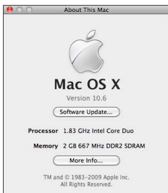
Figure 3-1: The About This Mac window identifies the processor type and version of Mac OS X.
