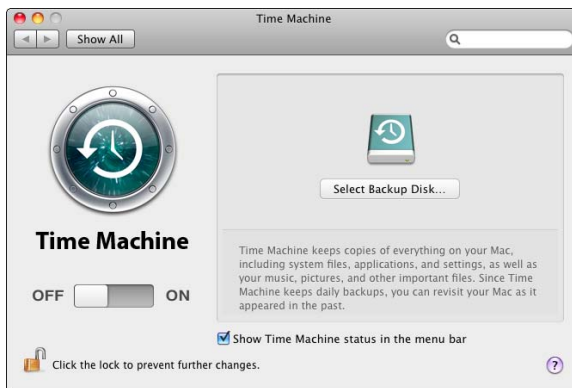
Figure 2-2: To set up Time Machine, you need to turn it on and choose an external drive to use.
