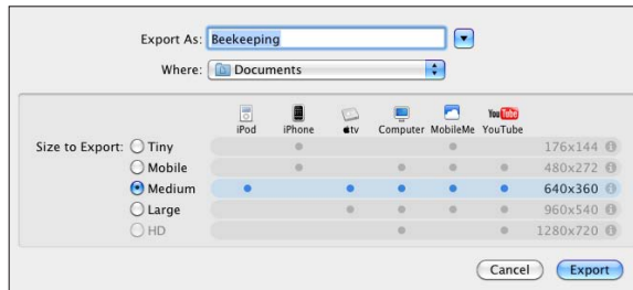
Figure 2-15: The Export Movie dialog lets you choose the resolution for playing on different devices.
