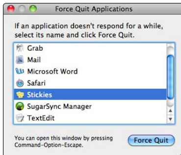
Figure 5-1: The Force Quit Applications dialog lets you choose a program to force-quit.
