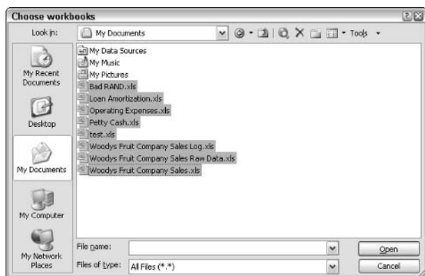
• Figure 68-10: The GetOpenFilename command opens this dialog box onscreen, allowing you to choose multiple files.
