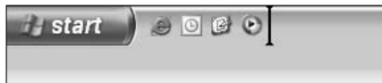
• Figure 2-4: The thick, black line indicates where Windows will drop your application.
