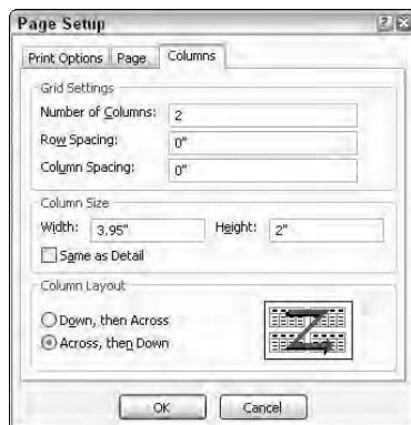
Figure 1-25: The Columns tab of the Page Setup dialog box defines how your report prints on sheets of labels.
