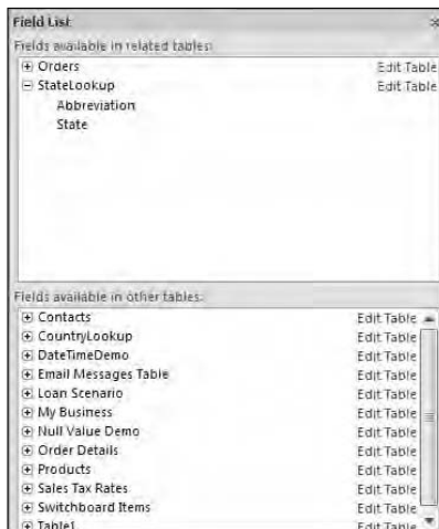
Figure 1-7: The Field List displays existing fields categorized by related tables and other tables.
