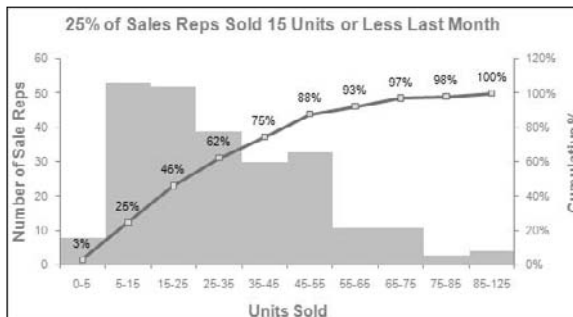
Figure 8-14: The cumulative percent series shows the percent of the population that fills all the Bins up to each point in the histogram.
