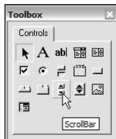
Figure 16-3: You use the tools in the Toolbox to add controls to a UserForm.
