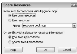
Figure 4-31: Use this dialog box to disconnect a project from the resource pool.
