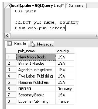
Figure 4-6: Using the SELECT statement to select specified columns from a single table.
