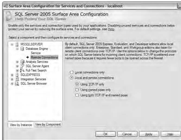
Figure 17-2: The Surface Area Configuration for Services and Connections dialog box, showing where you can specify whether remote connections are allowed.
