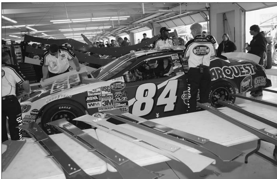
Figure 5-2: NASCAR inspectors fit templates to a car during inspections.
