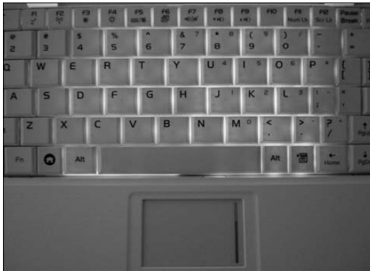
Figure 23-1: Light shines up through the spaces between keys, backlighting the keyboard.
