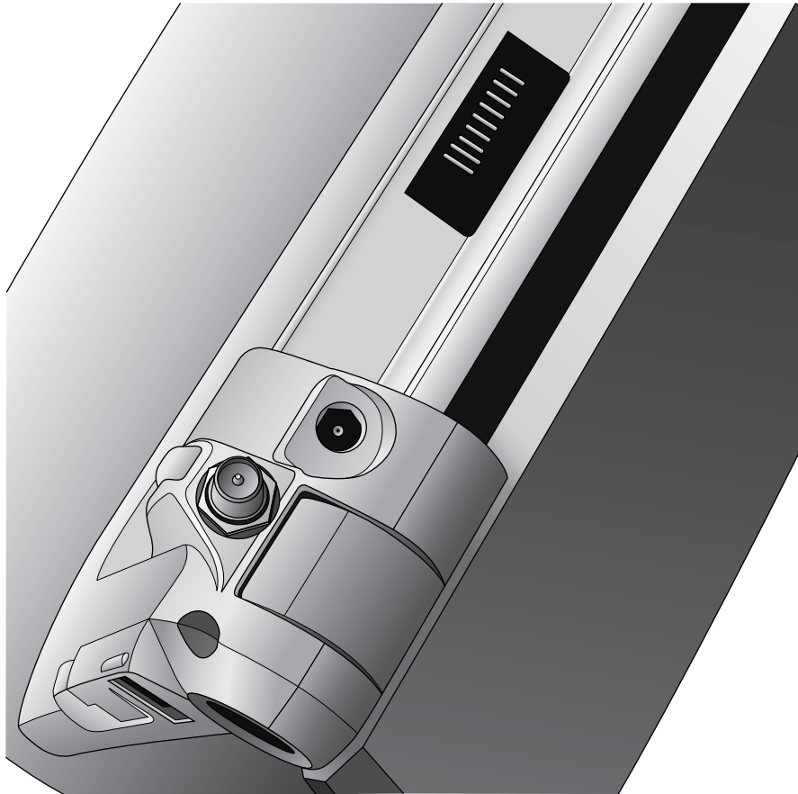
Figure 23-6: An Eee PC with an added external Wi-Fi antenna jack.
