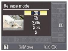
Figure 2-14: You can change the Release mode via the Quick Settings display.
