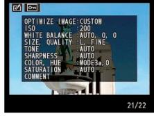
Figure 4-9: You can view the camera settings used to capture the image in Shooting Data display mode.
