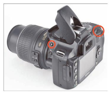
**Figure 2-5**: To change the flash mode, rotate the Command dial while pressing the Flash button.
