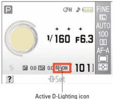
Figure 5-19: Press the Active D-Lighting button while rotating the Command dial to turn the feature on and off.
