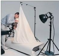
Figure 7-19: Investing in a light cube or tent makes photographing reflective objects much easier.
