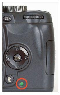
Figure 2-4: The memory card access lamp lights while the camera sends the picture data to the card.
