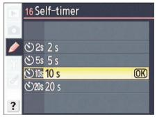
Figure 2-13: You can adjust the self-timer capture delay via the Custom Setting menu.
