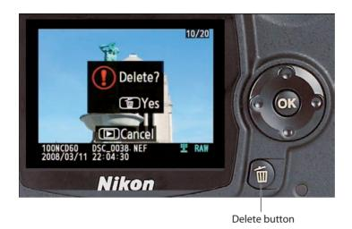
Figure 4-13: Press the Delete button to display this confirmation screen; press again to dump the picture for good.
