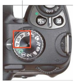
Figure 5-1: You can control exposure and other picture properties fully only in P. S. A. or M mode.
