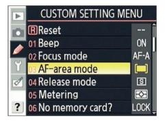
**Figure 6-4**: The AF-area mode control is also found on the Custom Setting menu.
