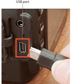
Figure 8-3: The USB slot is hidden under the little rubber door on the left rear side of the camera.
