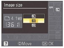
Figure 3-5: The Image Size control is positioned at the top of the Shooting Info display.
