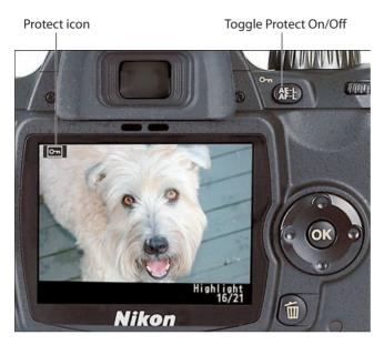
Figure 4-16: Press the AE-L/AF-L button to prevent accidental deletion of an image.
