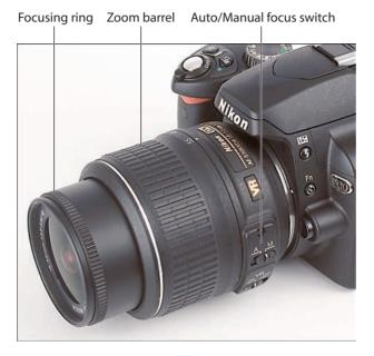
Figure 1-3: Set the focusing mode switch to M before turning the manual focus ring.
