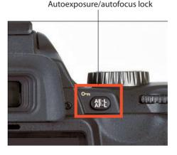
**Figure 6-9:** Press the AE-L/AF-L button to lock focus when using autofocusing.
