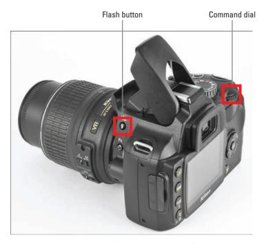
Figure 5-29: Hold down the Flash button and rotate the Command dial to adjust the flash mode.
