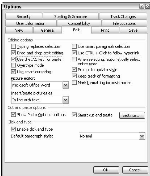
• Figure 66-1: Tell Word to use the Insert key for pasting instead of wiggling out to overtyping mode.
