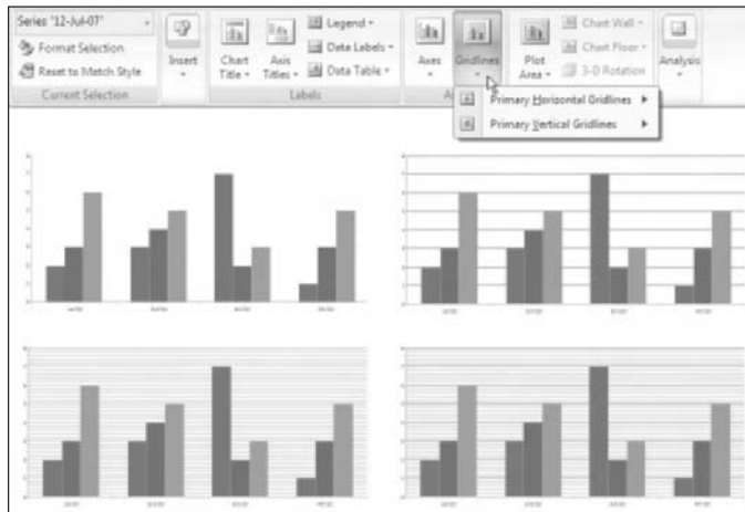
Figure 6-7: Options for handling gridlines (clockwise from upper left): None, Major Gridlines, Major & Minor Gridlines, and Minor Gridlines.
