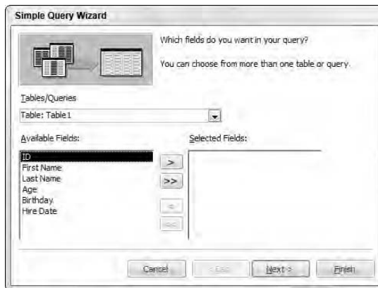
Figure 17-9: The Simple Query Wizard dialog box lets you pick the fields to use for your query.
