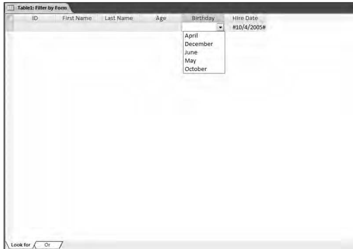
Figure 17-4: Filtering by form lets you choose the type of data you want to view from a pull-down menu.
