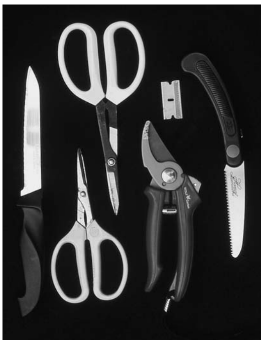
Figure 3-1: Cutting tools — from left to right: thin knife, two pairs of scissors, bypass hand pruners, single-edge razor blade, and folding pruning saw.
