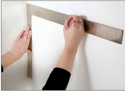
Figure 3-1: A square checks that items (such as holes for drilling) are at a right angle to an adjacent wall, surface, or straight edge.
