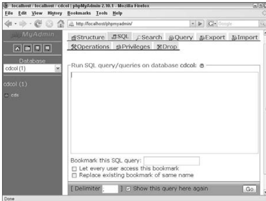
Figure 1-3: The phpMy Admin page that allows you to type an SQL query.
