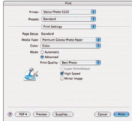
Figure 14-10: Select Media Type and Best Photo in the Print Settings dialog box.
