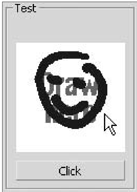
• Figure 12-8: Doodle in the Test area to make sure that the pressure sensitivity setting is right.
