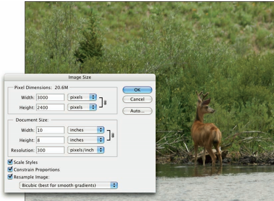
Figure 2-5: At the top, real information about your image. Below, merely printing instructions.
