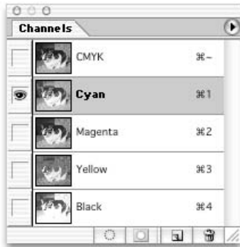
Figure 20-2: Photoshop's Channels palette presents conclusive evidence that color channels exist. Here the Channels palette is displaying the channels for an image in CMYK color mode.
