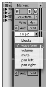
Figure 1-1: Select a view of a region in a track from the Track View menu.
