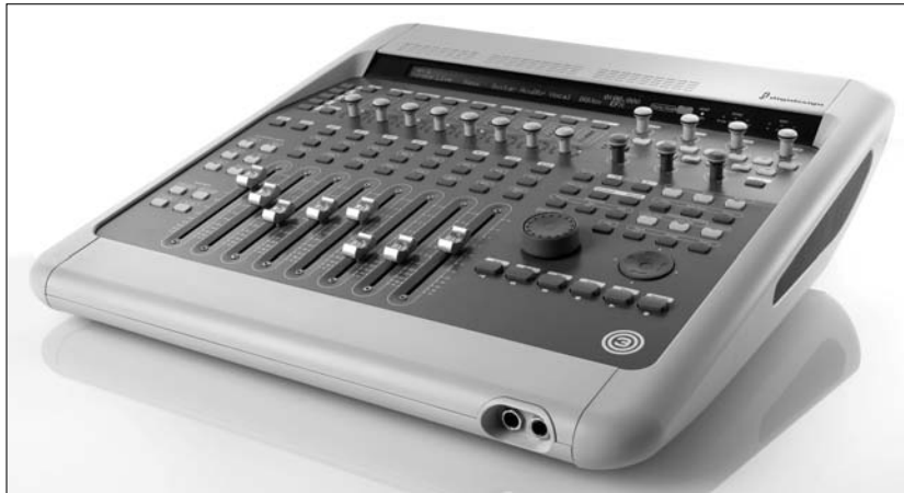
Figure 2-5: The Digi 003 has a full-function control surface as well as a FireWire interface.
