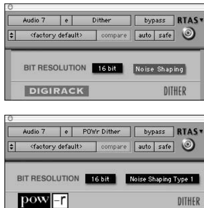
Figure 2-2: Pro Tools comes with two dithering plug-ins: Dither (top) and POWr Dither (bottom).
