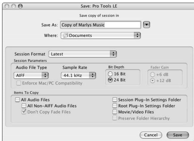
Figure 3-8: The Save Session Copy In dialog box allows you to change the type of file your session is formatted in.
