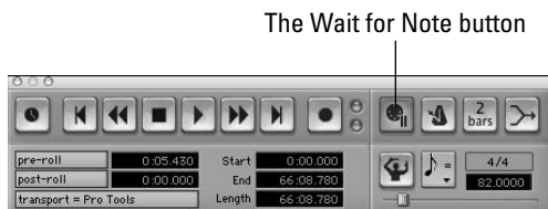
Figure 2-1: Engage Wait for Note to start recording the instant a MIDI note is received.
