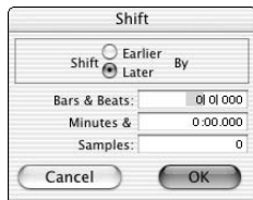
Figure 4-11: Use the Shift dialog box to adjust for the latency of the Mbox.
