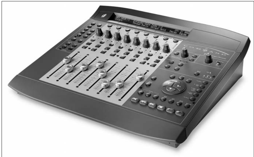
Figure 1-6: A computer control surface offers you real knobs and faders and still uses the mixer that's part of your Pro Tools software.
