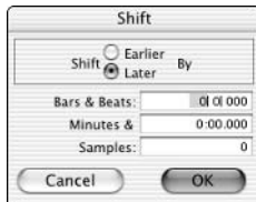
Figure 4-13: Use the Shift dialog box to adjust for the latency of the M-Box.
