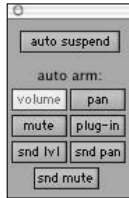
Figure 6-3: The Automation Enable window.
