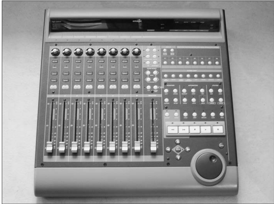
Figure 1-6: A computer control surface offers you real knobs and faders and still uses the mixer that's part of your Pro Tools software.
