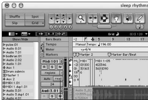
Figure 6-1: Access the five Pro Tools automation modes using the Automation selector in the Track Control section of the Edit window.
