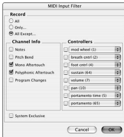
Figure 1-4: The MIDI Input Filter dialog box lets you choose MIDI parameters to record along with your performance data.
