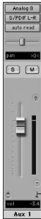
Figure 4-31: The Auxiliary Track channel strip is used for effects sends, sub-mixes, and monitor mixes, among other things.
