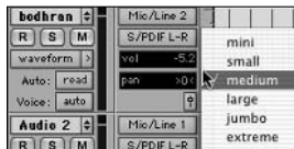
Figure 1-3: Open the Track Height menu by clicking the far-right edge of the Track Controls section.
