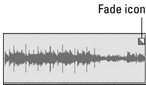
Figure 4-5: To get the Fade icon, put the cursor in the upper half near the Start or End point.
