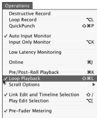
Figure 4-8: Checking the Loop Playback under the Operations menu to create a loop.
