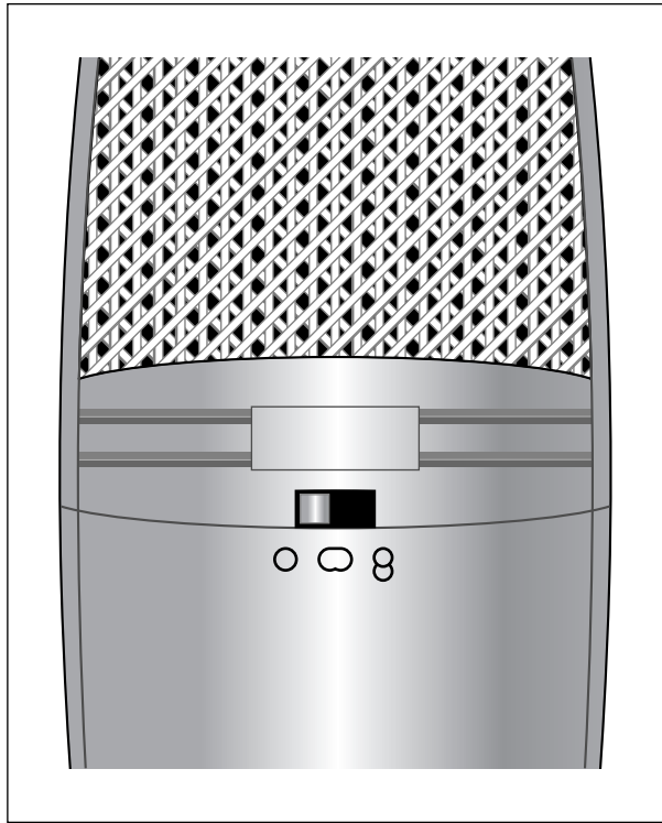
Figure 5-8: Some mics have a switch that allows you to change polarity patterns.
