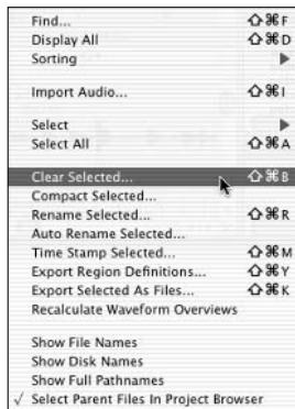
Figure 4-22: Choosing Audio Regions ⇨ Clear Selected from the main menu gets rid of a selected take.
