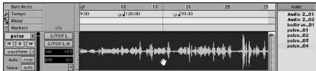
Figure 4-15: Use the Grabber tool to select the take you want to replace.
