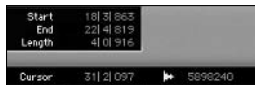
Figure 4-20: The Cursor display tells you the location of the cursor in the session.
