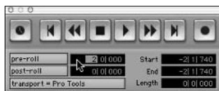
Figure 4-4: Clicking the Pre-Roll or Post-Roll field lets you enter a value for the pre/post roll.
