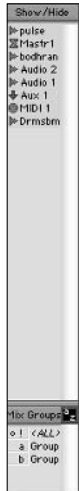
Figure 4-37: The Show/Hide Tracks list and Groups list allows you to organize your tracks in the Mix window.
