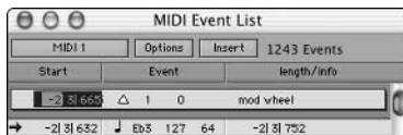
Figure 3-17: The Controller Event entry window has fields for the start time, controller number, and value.
